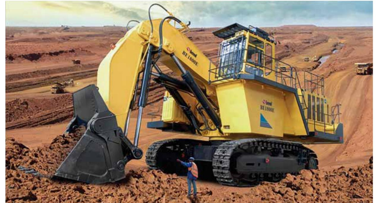
▲ BEML180 ton Electric Hydraulic Excavator BE 1800E is the largest excavator available.
