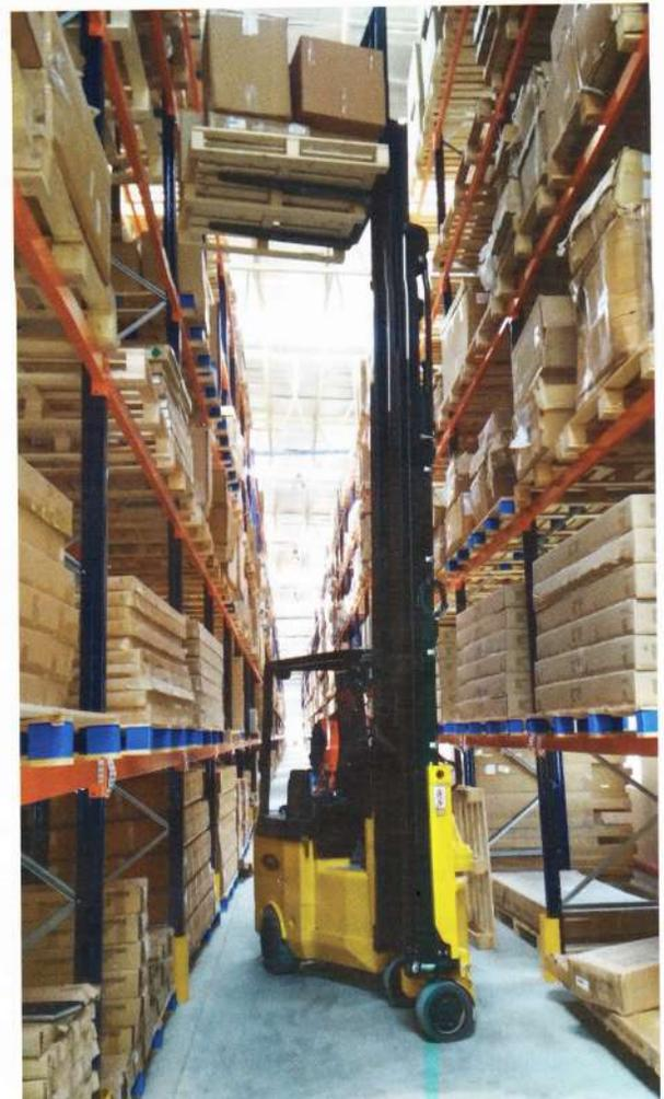
▲ Articulated Truck working in narrow working aisles
